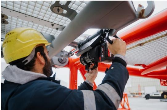
Caption: Battery-powered bolt pulling cylinder in use
